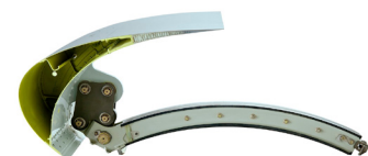
Slat Track SLATS are the aerodynamic surface on the leading edge of the wings of aircrafts which allow the wing to operate at a higher angle of attack, thereby increasing lift, which results from the combination of the angle of attack and speed.
