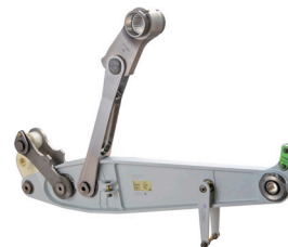
Droop nose for the Airbus A380 Length: 1,000 mm
